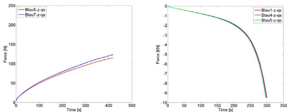
**Figure 3: Quasistatic tensile testing (left) and compressive testing (right)**
