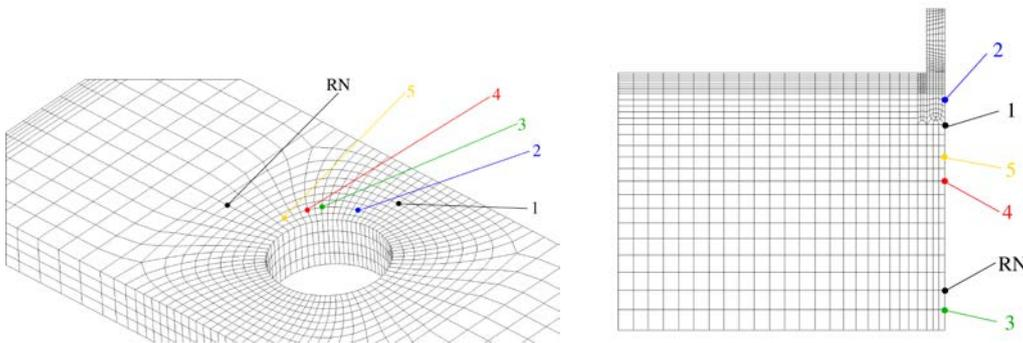
**Figure 9:** Position of the relative node and the verification nodes on the FE model of the tensile and compressive test specimens.
