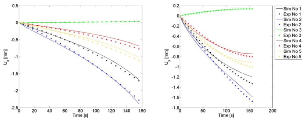
**Figure 10: Relative measured and simulated radial and longitudinal displacements for selected identification nodes, quasistatic compressive testing**
