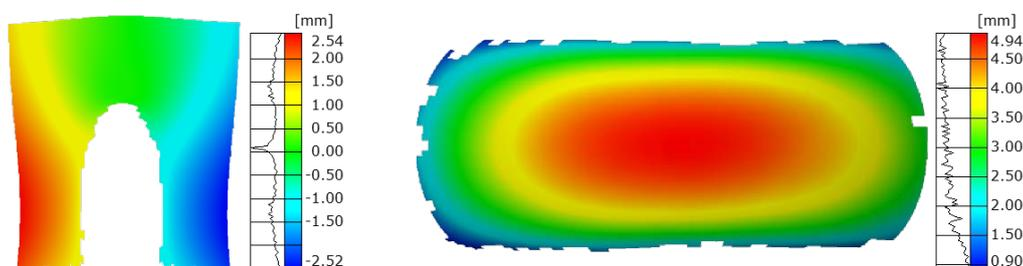
**Figure 6:** Displacement fields, tensile and compressive testing
