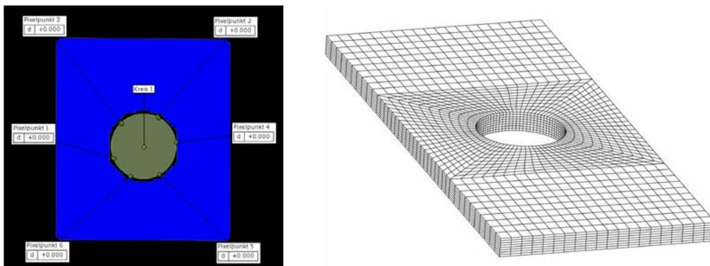
Figure 8: Transformed coordinate system and FE model (examples)
