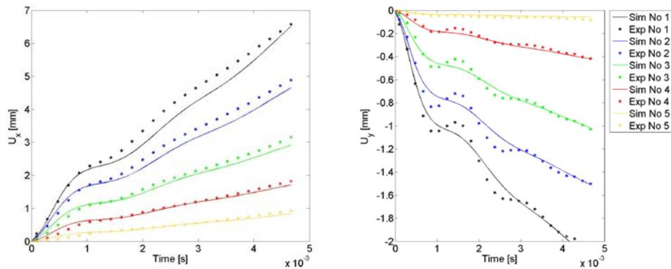
**Figure 13: Relative measured and simulated longitudinal and transverse displacements for selected identification nodes, tensile testing at 5.0 m/s**
