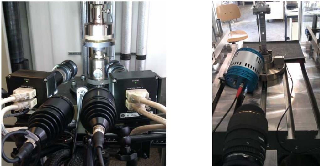
**Figure 1: Quasistatic compressive test, high-speed tensile test**
