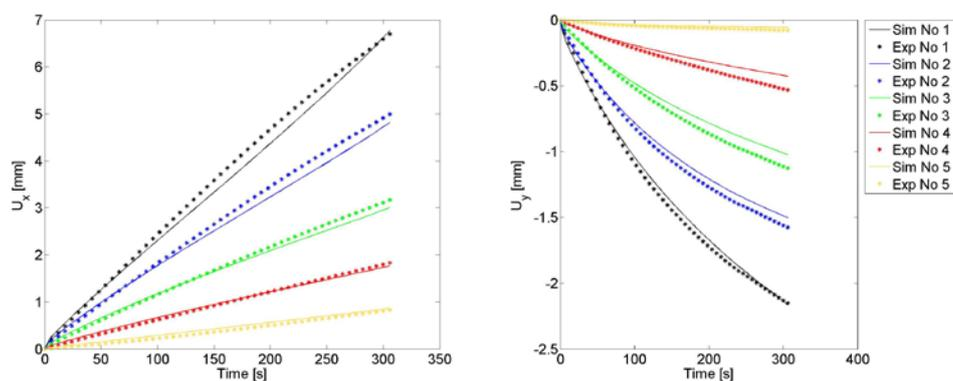
**Figure 11: Relative measured and simulated longitudinal and transverse displacements for selected identification nodes, quasistatic tensile testing**
