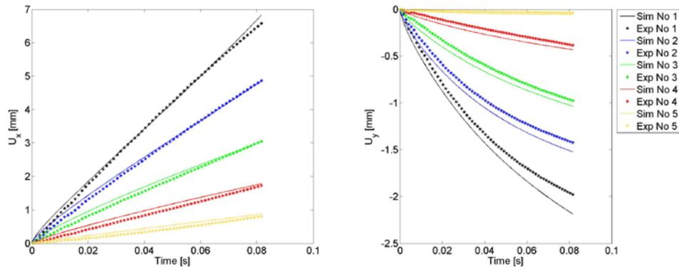
**Figure 12: Relative measured and simulated longitudinal and transverse displacements for selected identification nodes, tensile testing at 0.3 m/s**
