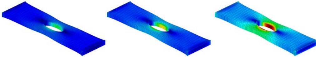
**Figure 14:** Stress distribution at a quasistatic load (left), at 0.3 m/s (middle), and at 5.0 m/s (right)
